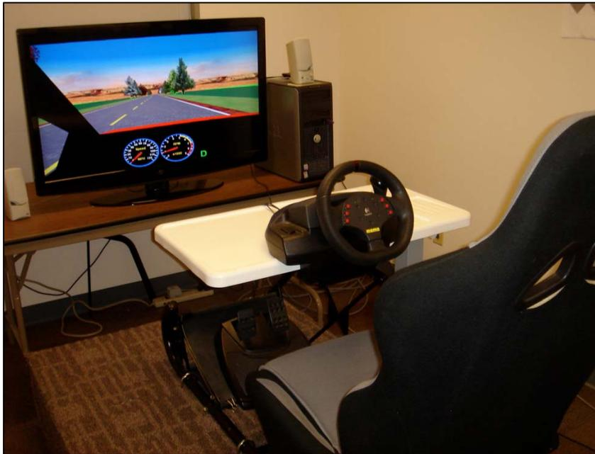
Figure 1. Experimental setup using a System Technologies, Inc., STISIM Drive, build 2.08.10, a Westinghouse 42-inch LCD monitor and Logitech MOMO racing force feedback wheel.
