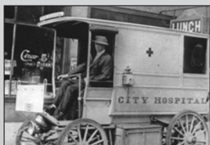
Ambulance Driver Nick Palucci is shown driving the 1912 Electric Winton. It was the first motorized ambulance with a top speed of 20 MPH, and a foot powered gong for clearing traffic.
